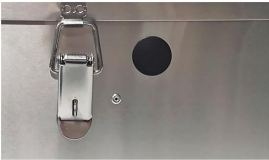
Remove the nut from the photo cell.
