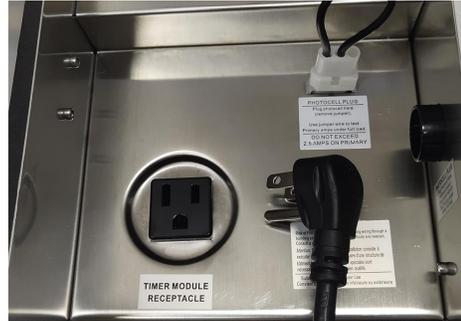
Insert that plug into the side of the timer as shown. Insert the timer into the outlet on the transformer as shown.
