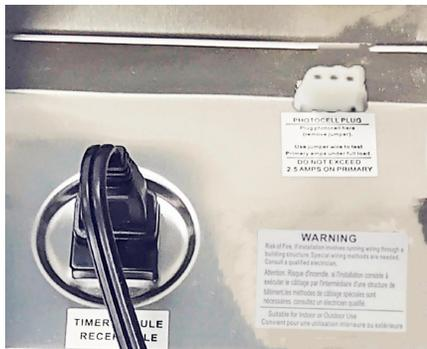
Insert the wire and connector of the photo cell through the hole in the side of the transformer. Place the nut around the wire and screw onto the photo cell, holding the unit in position.
