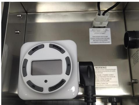
Follow the instructions for the timer to set the clock and on and off times or manually turn on/off your system.
